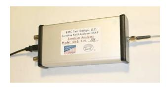
Spectrum Analyzer SA-S is equipped with powerful RF signal processing software, preprogrammed with OFA-S antenna factors, allowing the display of the measurement data in natural field strength or power density units.
