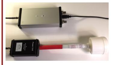
**USB Spectrum Analyzer** is equipped with powerful RF signal processing software, preprogrammed with OFA-GH antenna factors, allowing the display of the measurement data in natural field strength or power density units.
