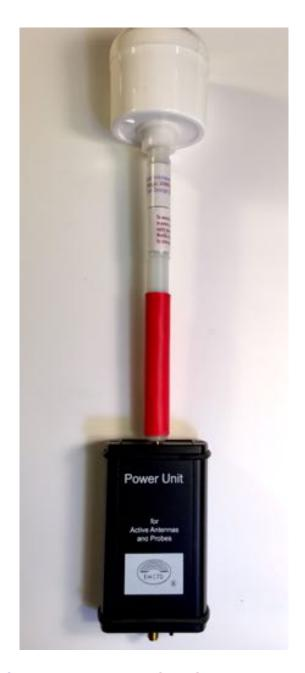
Omnifield Antenna® OFA-GH consists of antenna head with handle and detachable power unit PU-5G.
